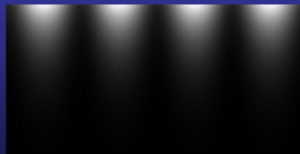
Excitation of two surface plasmons and generated interference pattern
