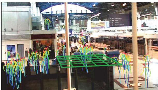
Fig. 6. Example of visualized pose detection used for camera parameters estimation (PETS 2006, camera 2). The ground plane computed with the predicted calibration parameters is shown in green (each square side is 1 m). The assumption of a single ground plane is violated by the human detection on the balcony. False detections are also present (note the big figure in the middle and the figure on the balcony), however the estimated ground plane is quite plausible
