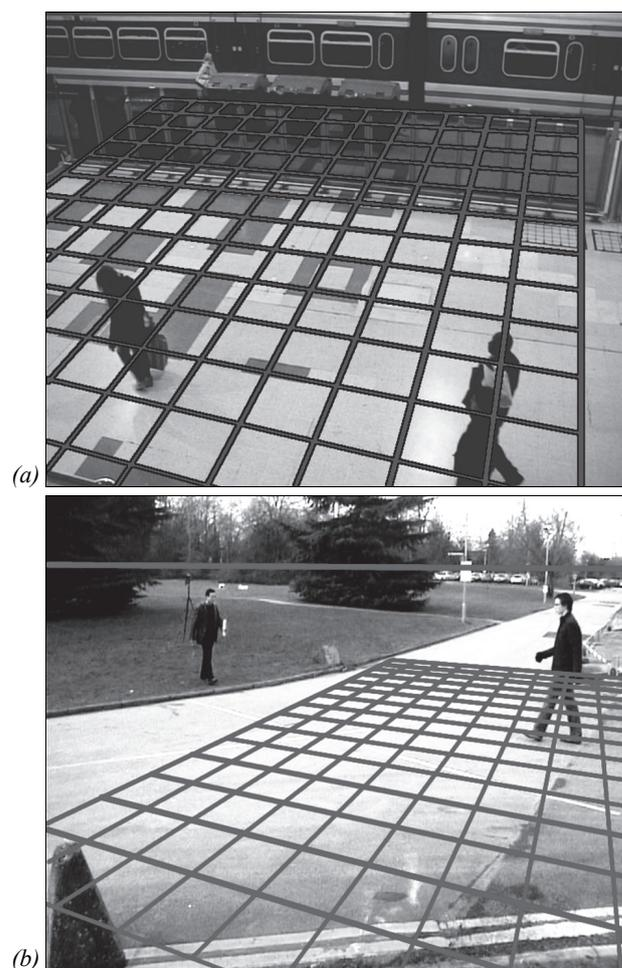
Fig. 8. Visualization of the ground plane (shown as a grid; each square side is 0.5 m) computed with the predicted calibration parameters for two PETS videos
