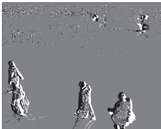
Fig. 7. A visualized frame of simulated event-based stream for one of PETS 2006 sequences
