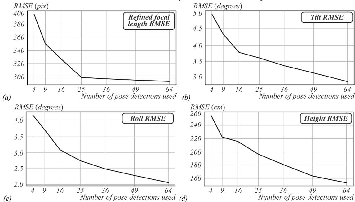
Fig. 5. RMSE for various input detections number: (a) focal length RMSE; (b) tilt RMSE; (c) roll RMSE; (d) height RMSE
