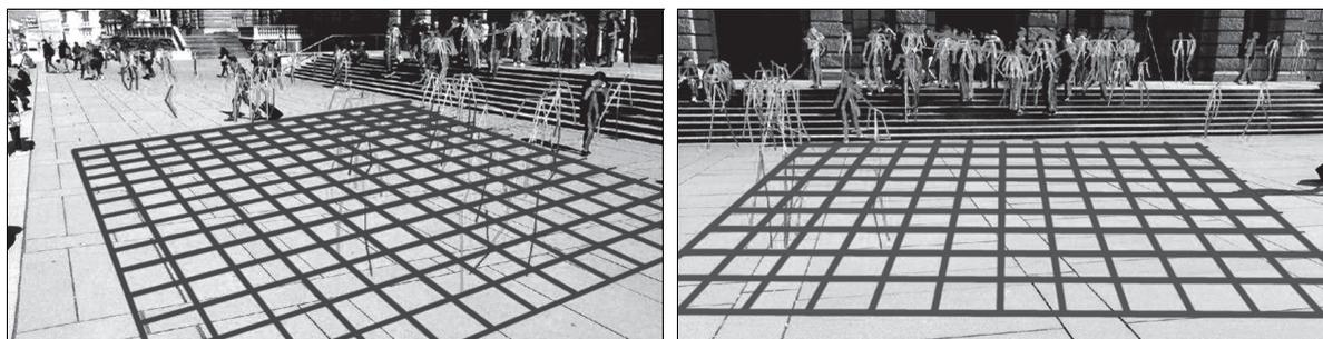
Fig. 9. Visualization of the ground plane (shown as a grid; each square side is 0.5 m) computed with the predicted calibration parameters for videos with detections that violate the assumption of a single ground plane
