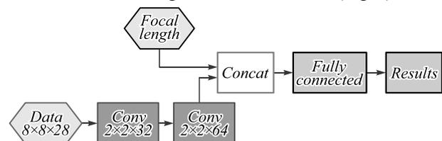
Fig. 3. An architecture of the proposed network estimating extrinsic parameters (LON)
