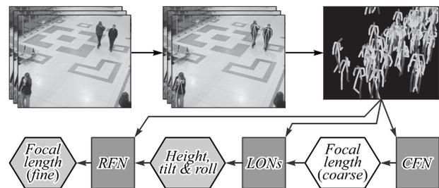
Fig. 2. The scheme of the proposed method. Rectangular boxes depict neural networks. Arrows show CNNs inputs and outputs
