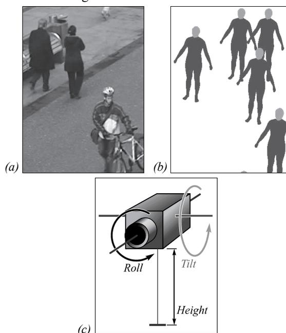
Fig. 1. (a) A part of the CCTV scene; (b) scene geometry can be estimated just from detected human positions and scale without any background information; (c) extrinsic camera parameters
