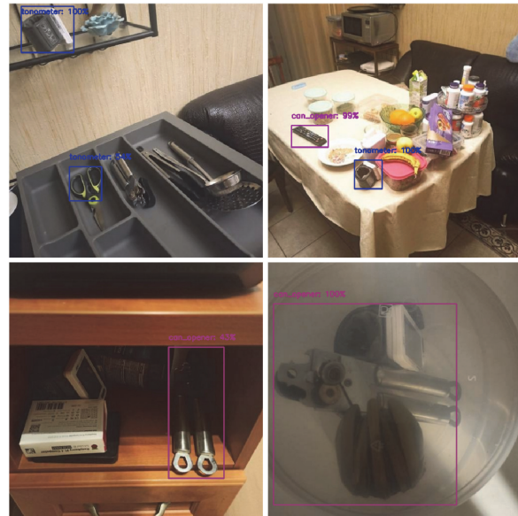
Fig. 3. Examples of incorrect detections on test data with int8 quantized EfficientDet for 320x320 model size
