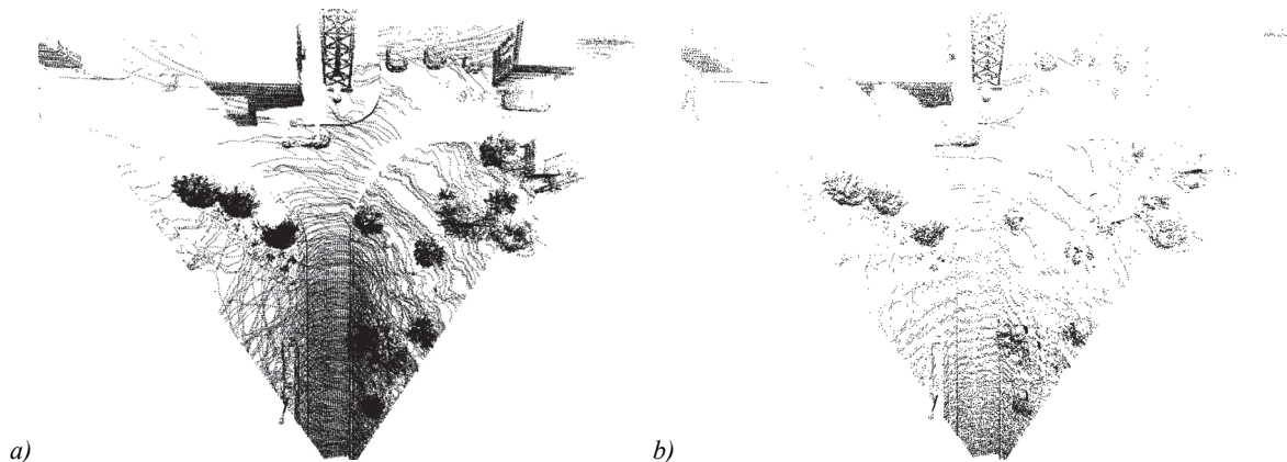
Fig. 4. Visible point cloud extraction: (a) Points in camera frustum; (b) Visible point cloud
