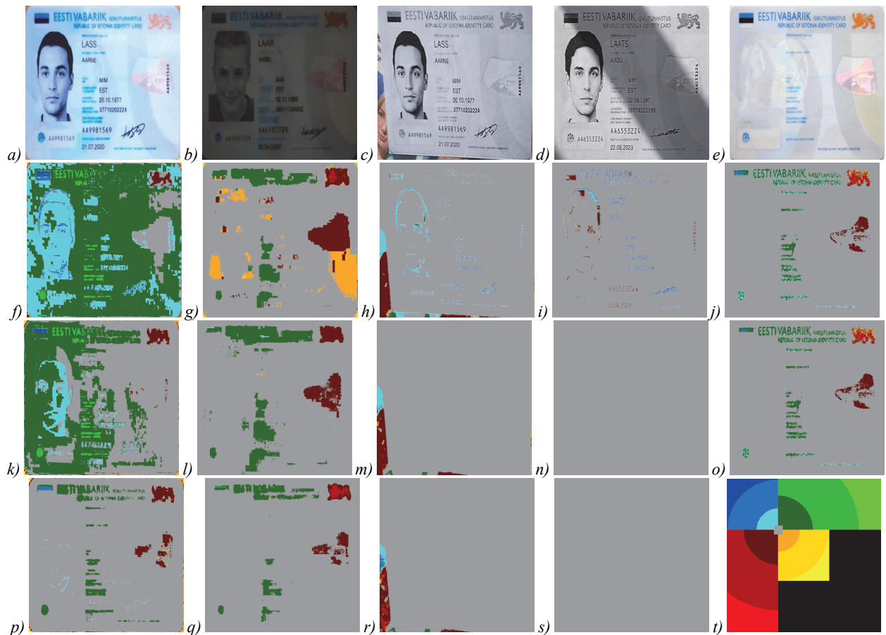
Fig. 5. An example of a chromaticity distribution changing for input images: (a)-(d) input document images in question, (e) input template image, (f)-(j) the chromaticity distribution of input images, (k)-(o) the chromaticity distribution of input preprocessed images, (p)-(s) the chromaticity distribution of input document images after histogram matching. The colors of pixels for images (f)-(s) correspond to some color from the color schema (t) depending on the chromaticity values
