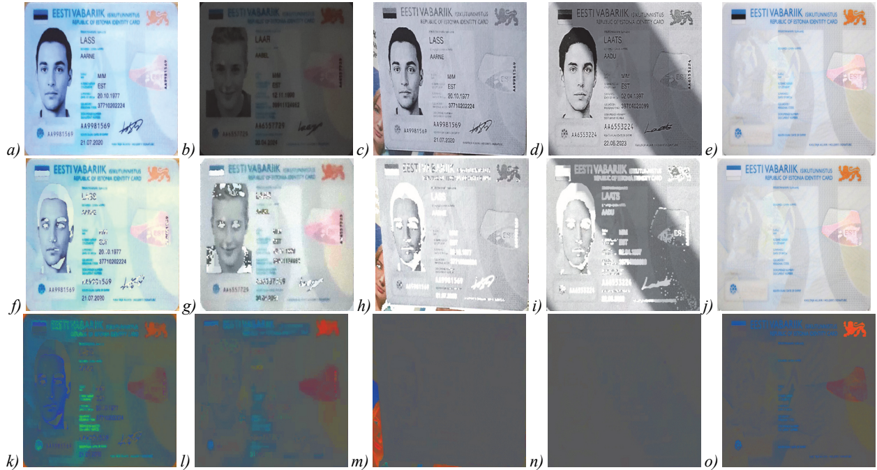
Fig. 3. The preprocessing steps for input images: (a)–(d) input document images in question, (e) document template, (f)–(j) the result of the sequential contrasting, filtering “dark” pixels and color normalization, (k)–(o) the result of the input image processing (for the convenience of visualization, the saturation of (k)–(o) was tripled)
