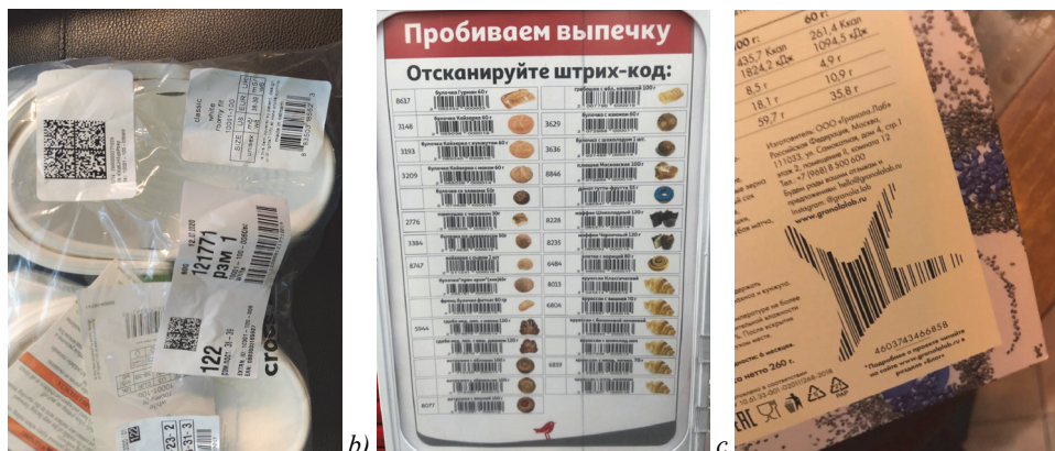
Fig. 1. Examples of complex code detection cases: a) several barcodes of different types and shapes with projective distortions; b) densely spaced linear codes; c) "designed" code
