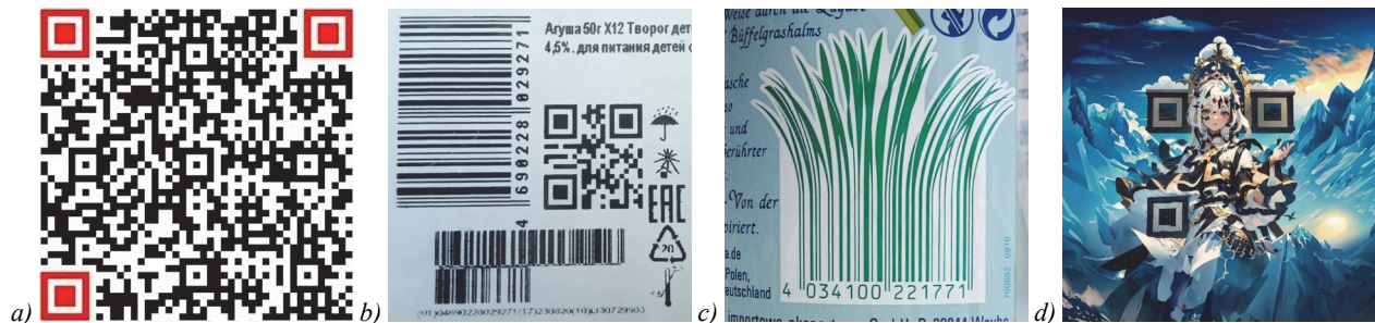
Fig. 2. Real barcode usage samples: (a) “finder patterns” of QR code type, (b) many barcodes of different types in a small area, (c) “designed” code sample in complex background, (d) “designed” QR code generated via Stable Diffusion
