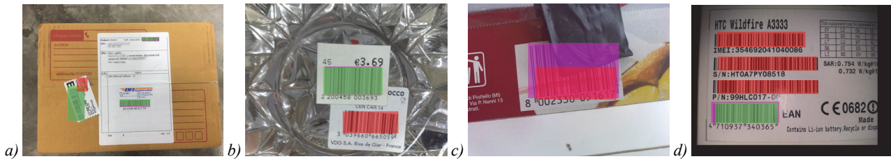
Fig. 7. Detection results of the YOLO-Barcode on Muenster, ArTeLab and ParcelBar datasets. (a) ParcelBar, small barcodes on the complex background, (b) ArTeLab, big barcodes on the simple background, incorrect GT, (c) MuensterDB, partially closed barcode, (d) ArTeLab, many long-shaped barcodes, incorrect GT. Magenta denotes ground truth, green – correct detection result, red – false positive answer
