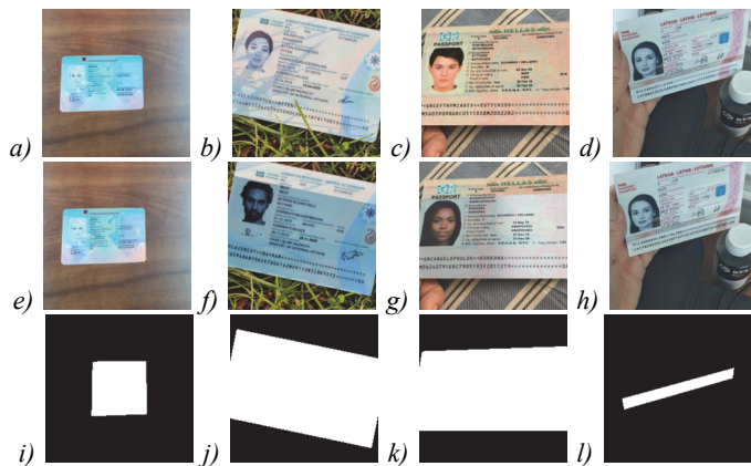
Fig. 5. Examples of gluing from MIDV-DM: (a)–(d) – genuine images, (e)–(h) – corresponding forged images, (i)–(l) – corresponding masks indicating the area of manipulation
