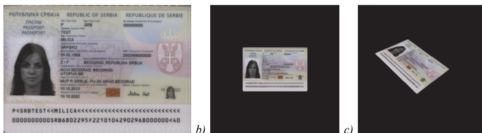
Fig. 4. The process of synthesizing document images with geometric distortions. (a) Ideal document, (b) Camera image, (c) Simulated distortion
