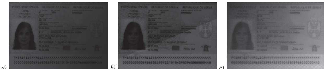
Fig. 5. Simulation of different lighting conditions. (a) Global and local darkening, (b) Shadow, (c) Local lighting
