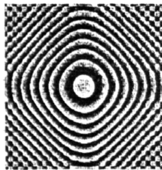
Fig.4 The phase of the focuser into a square obtained after 10 iterations from the initial geometro-optical phase.
